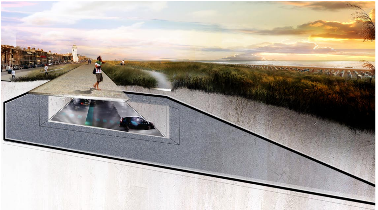
Top: subterranean parking garage in the dyke-in-dune Right: design with preferred coast reinforcement alternative
