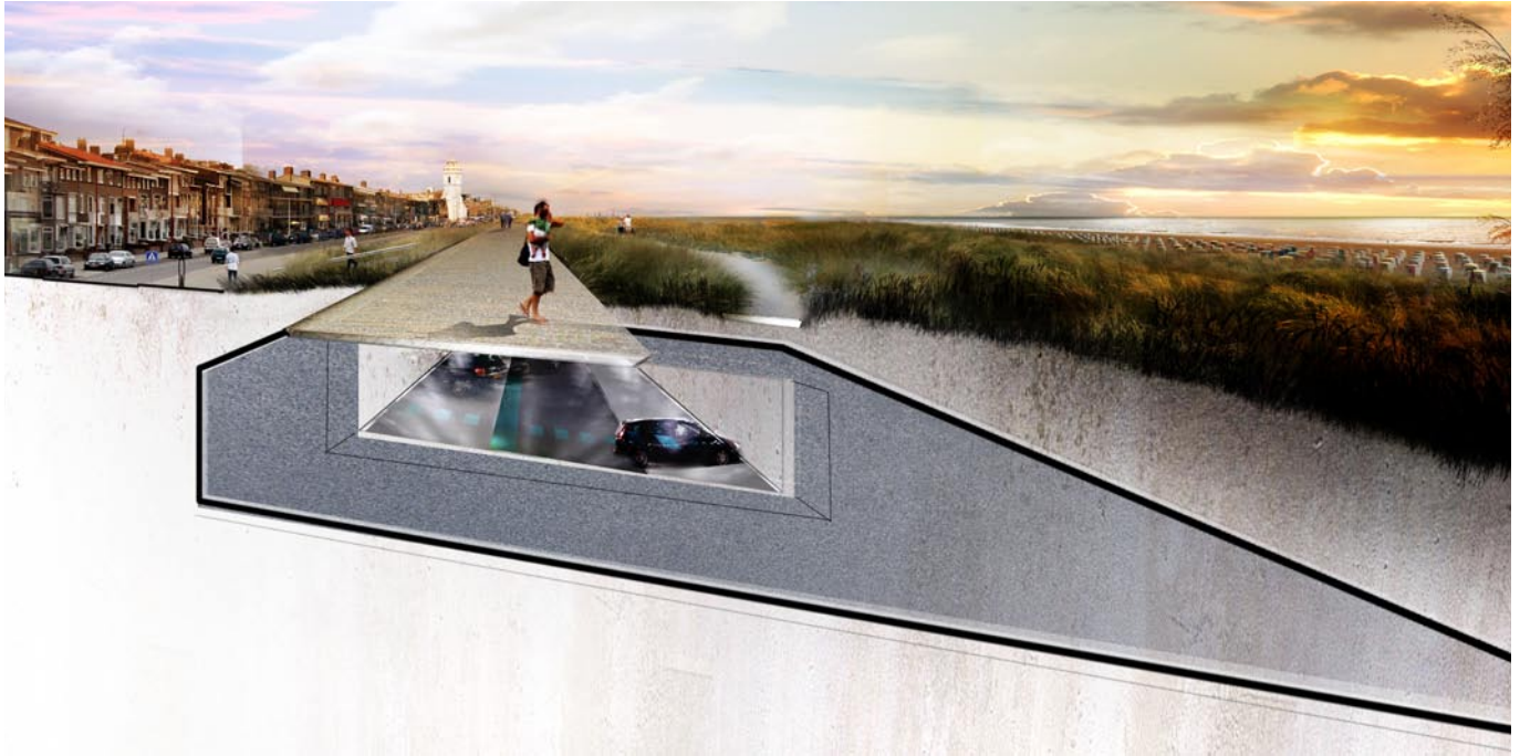
Visualization of the dyke-in-dune solution with an integrated parking garage, the chosen model.
